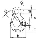
**Repair:** Eye Sling Hooks HS are only to be repaired by a qualified person. Damaged accessories must be replaced by new, original replacement parts. Welding, heat treatments, as well as the straightening of bent Eye Sling Hooks HS are not permitted. Inspections and repairs have to be documented and the corresponding reports have to be retained during the service life of the Eye Sling Hook HS.
