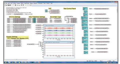
Using solidThinking Embed to develop the design models incorporating product requirements. Over two hundred individual dynamic block diagram based models were developed to capture the entire suite of requirements
