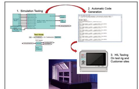
The verification process answers the question “did we build it right”. One way to answer this question is by Hardware In the Loop (HIL) testing the final product to confirm its performance complies with the specifications used to develop the requirements.
