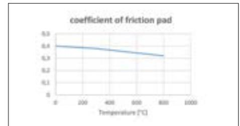
In a braking situation most of the kinetic energy is converted to heat causing a lower friction coefficient.
