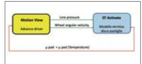
In the co-simulation, the line pressure and the wheel angular velocity is sent to the Activate model to determine the temperature and the related friction coefficient.
