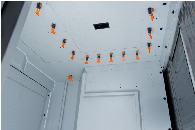
Fully enclosed machining zone with overhead shower wash for most efficient chip evacuation ▲
