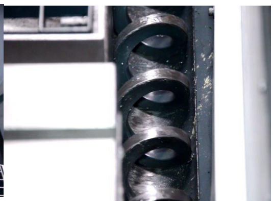
Screw Conveyor on both side of table for easy chip flow management ▲
