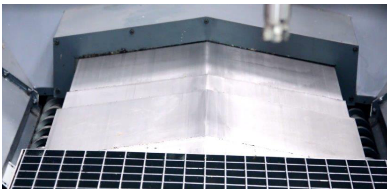
Screw Conveyor on both side of table for easy chip flow management ▲
