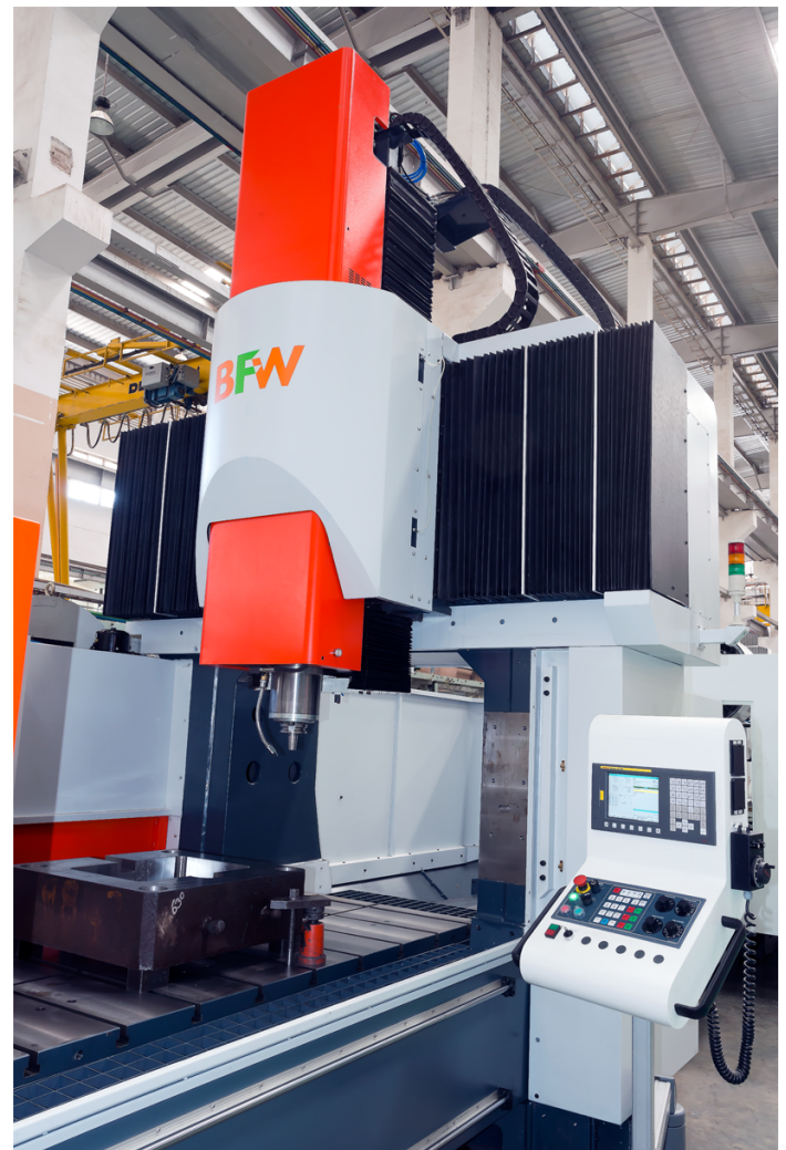
An exclusive design of moving RAM in Z-Axis increases the dynamic characteristics and ensures rigidity, stability and vibration free cutting, thus improving surface finish of machined components. ▲
