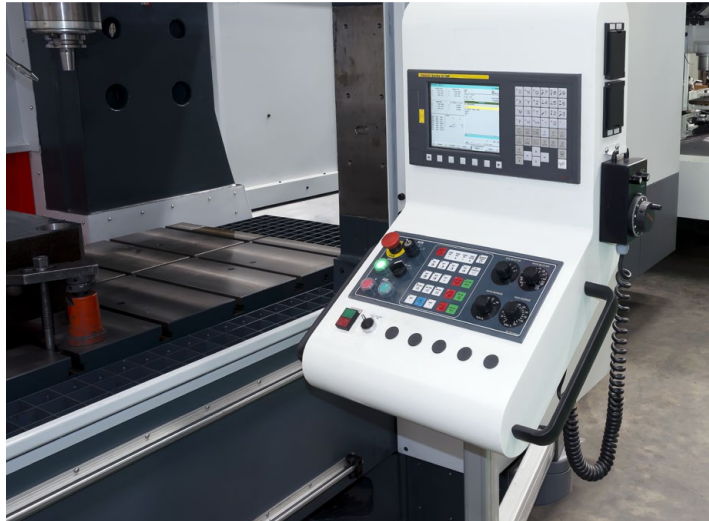
Operator panel with swing arm for easy accessibility to working area enabling better operator friendliness ▲
