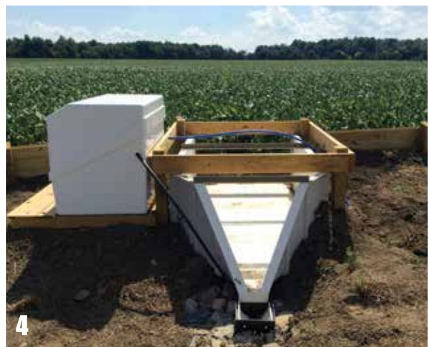
1. Area agricultural professionals get an up-close look at a sub-surface nutrient placement toolbar at Kellogg Farms. 2. Kevin King from USDA-ARS discusses how edge-of-field monitoring equipment takes water samples for later testing. 3. A blind inlet phosphorus filter bed being constructed on Kurt Farms. 4. Surface water flume for collecting samples for edge-of-field monitoring.
