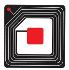
The RFID (Radio frequency identification) technology for contactless localization and recording of tangible assets uses electronic tags with built-in microchip instead of standard paper labels.
