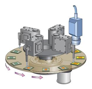
Ring Drives offer smooth motion, high load capacity and high speed. With their precision-grade, high-capacity cross-roller bearings, Ring Drives can handle loads up to 1,575 kilonewtons.
