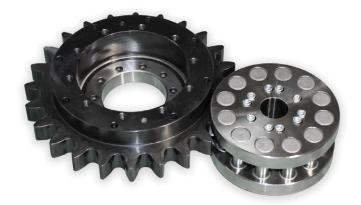
Nexen's Ring Drive System is based on the company's innovative Roller Pinion System (RPS) for linear motion. To create a Ring Drive, the linear rack becomes a circular gear. Instead of moving a linear rack side to side, the pinion rotates the gear. The pinion is equipped with bearing-supported rollers that engage a unique tooth profile in the gear, providing smooth rolling friction instead of sliding friction.
