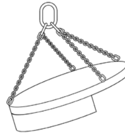
All the load is carried by one chain leg
