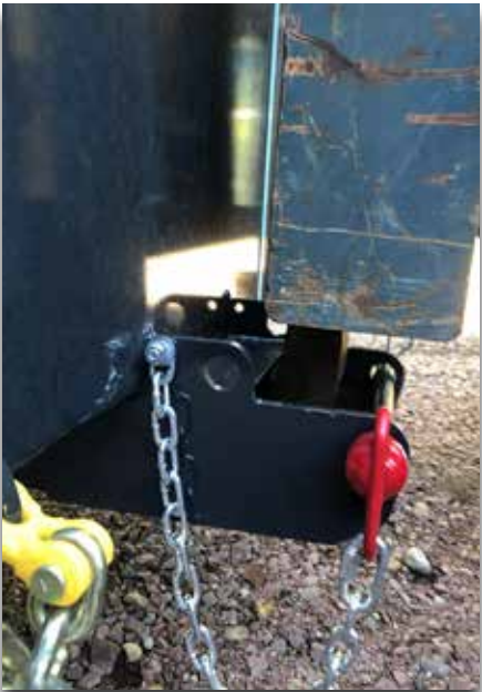
Secure mounting with two locking pins and secondary system with chain behind fork carriage frame.
