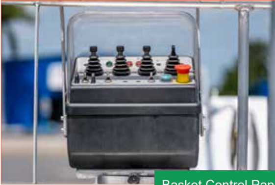
Basket Control Panel
