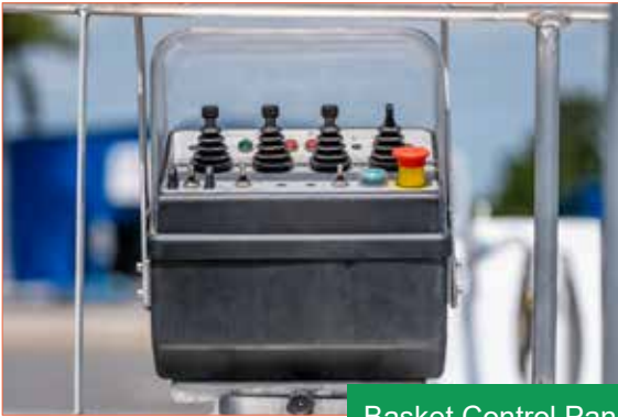
Basket Control Panel
