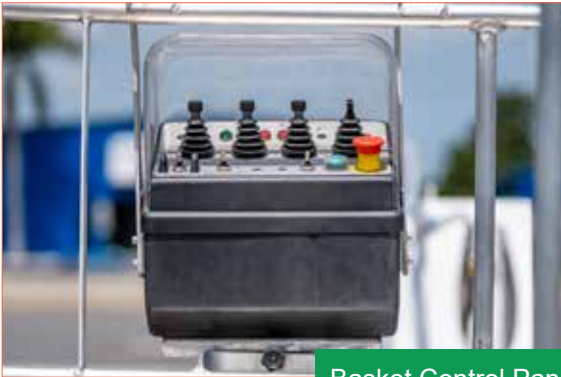
Basket Control Panel
