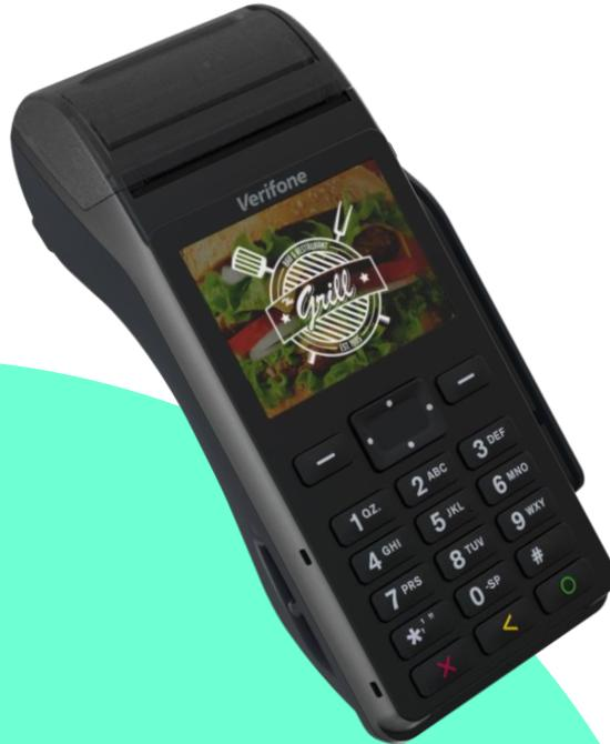
The Verifone V200t is an all-in-one, dual-function payment device that's designed to operate as a countertop solution via dial-up or Ethernet connectivity or as a portable payment solution with built-in battery and wireless radio functionality. As a member of the Verifone Engage family, the V200t combines features, functionality, and versatility to provide merchants the flexibility needed to run their businesses.
