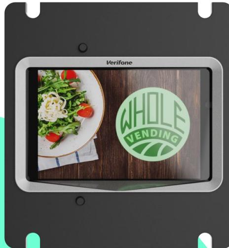
The UX115 works with other UX devices to meet self-service demands indoors and out. Featuring a bright, high resolution, color screen that helps guide the customer experience, the UX115 offers high performance and excellent durability. Its weatherproof construction is ideal for off-street parking meters, petroleum pumps, ticketing machines and more. Pair it with the UX300 or UX410 card readers to optimize your transaction functionality.
