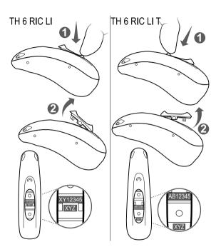
Note: If you press the lower part of the rocker switch more than 3 seconds, the hearing instrument may turn on. After reasembly you can turn off the hearing instrument by a long press to the upper part of the rocker switch.
