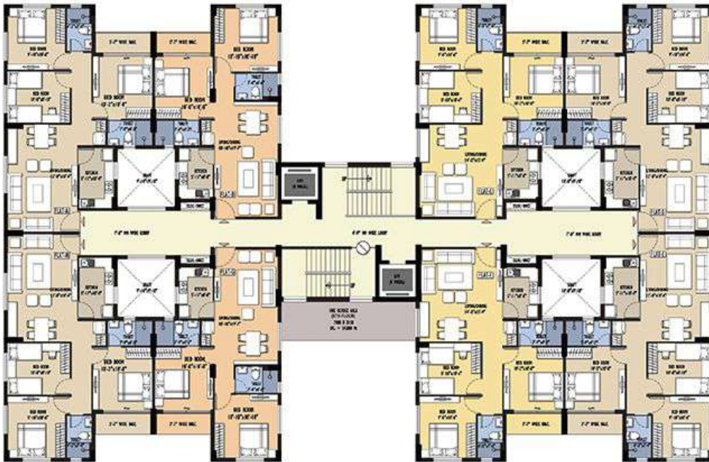
TYPE C - BLOCK 30 - 3RD TO 12TH FLOOR TYPICAL AREA PLAN
