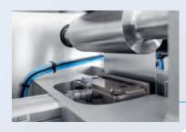
Patented internal and external pre-cut system adjustable with micrometer screws for V-Shapes® one hand unit-dose opening solution.
