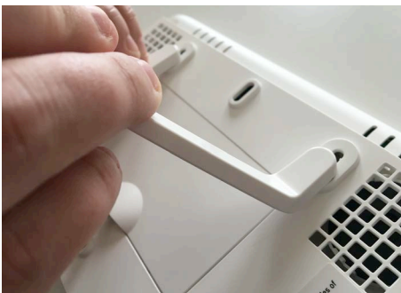
Insert the table stand into the mounting holes and push upward until it snaps into place
