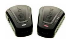
**Blue:** Sensor turned on, detected by software **Green:** Sensor plugged in, currently charging **White:** Sensor turned on, completed charging,
