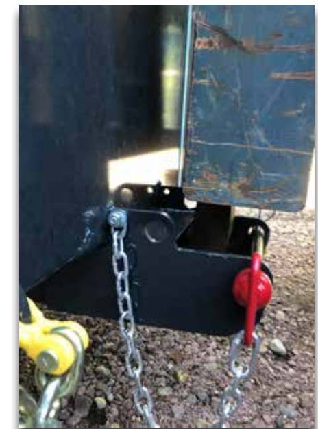
Secure mounting with two locking pins and secondary system with chain behind fork carriage frame.
